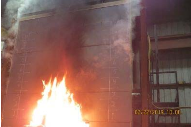
Photo No. 23 Smoke from wall during test
