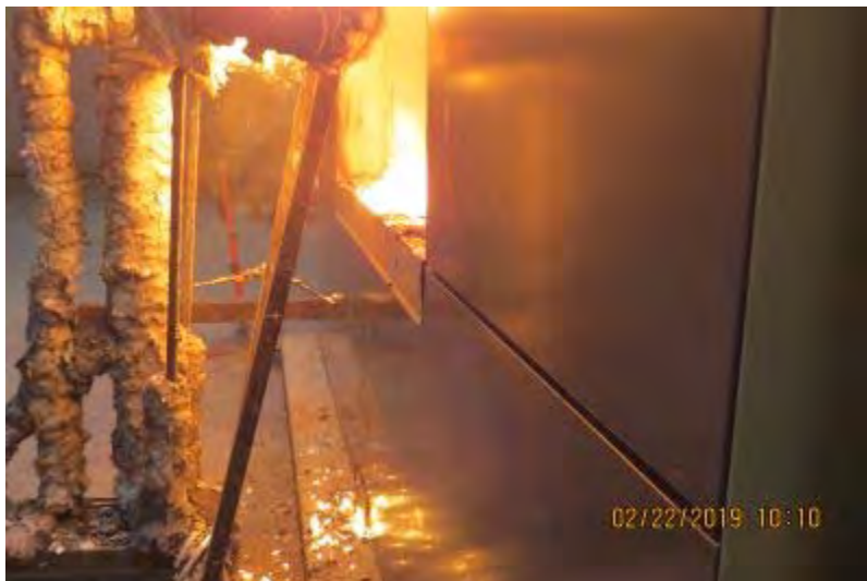
Photo No. 24 Flaming drops from panels above window opening
