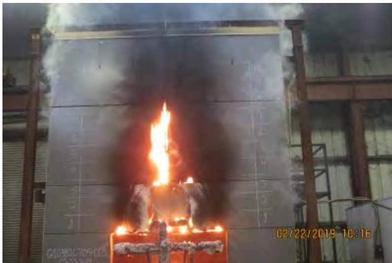
Photo No. 26 Burners turned off at end of 30-minute exposure
